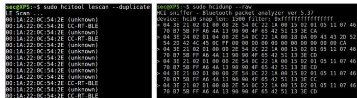
Fig. 28: Hcidump (*right*) running while scanning (*left*)
